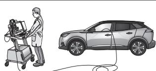
The light functions on the trailer will only operate **AFTER** the vehicle has been re-coded!
